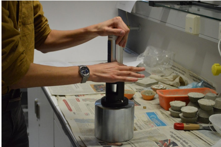
Student calibrating the concrete rebound test hammer PCE-HT-225A with the calibration block for concrete tester PCE-BPHC 1 at the European School of Frankfurt
