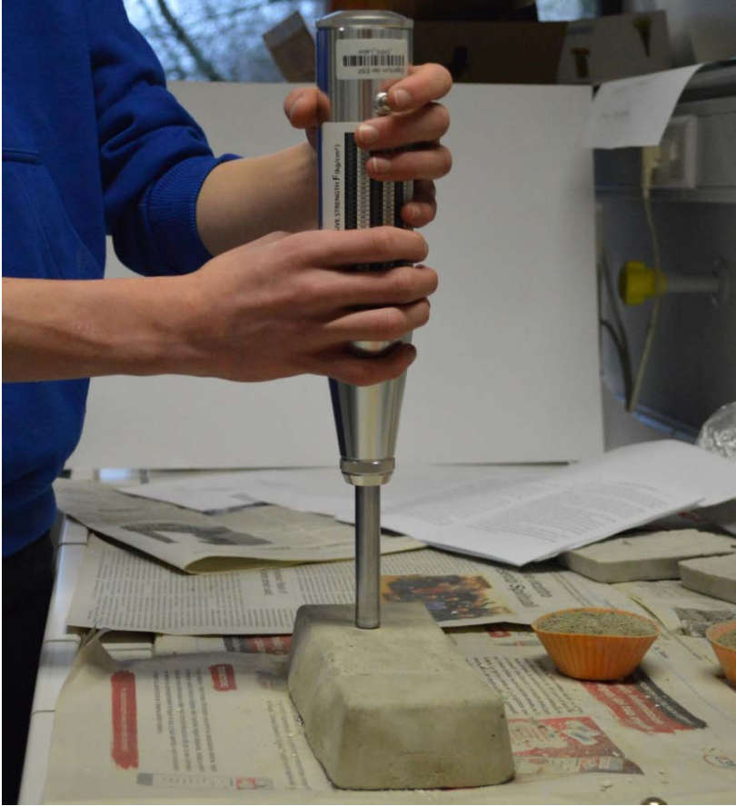
Student making a surface hardness and compression strength test on a sample brick with the rebound test hammer PCE-HT-225A
