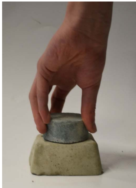
Student preparing the surface of a sample brick for the hardness and compression tests with the rebound test hammer PCE-HT-225A
