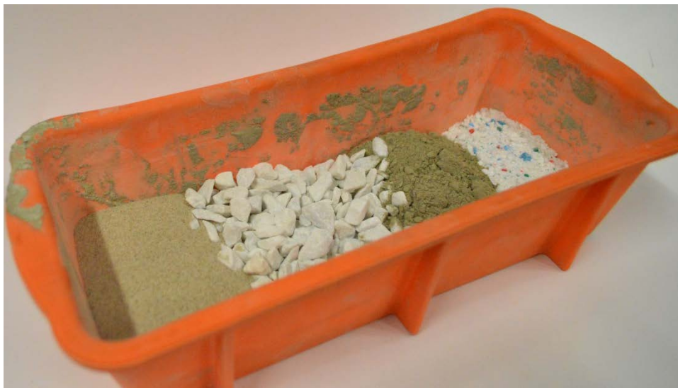
Materials used to make the sample bricks. From left to right: sand, aggregate, cement and plastic
