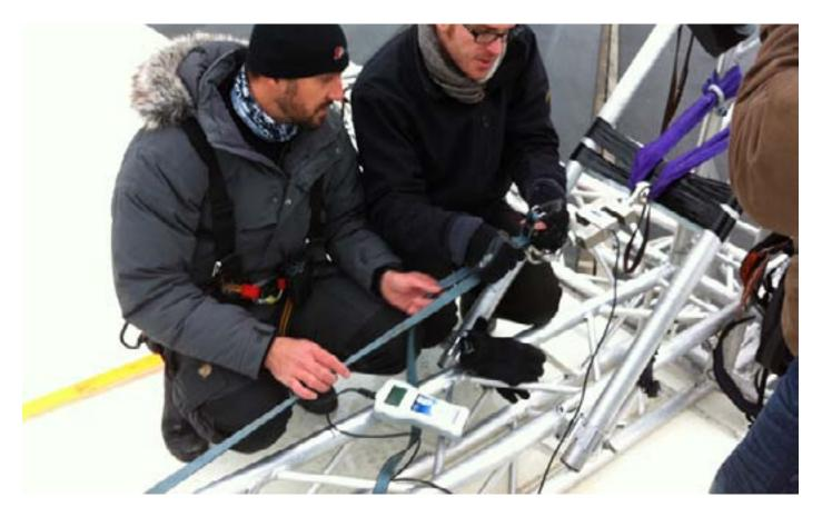
For safety reasons, the check was first carried out stationarily. The speed of the trucks was simulated by artificial wind. The wind strength was measured by means of the PCE-A420 anemometer, a digital cup anemometer with which the wind direction did not affect the measurement. Even stationarily, the stunt seemed to be impossible at 80 km/h as the wind pressure was enormous.
