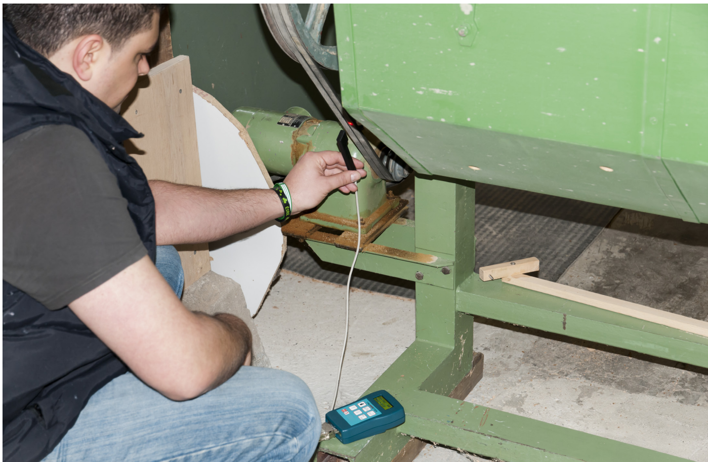
Instrument for use in belt tension mesurement
