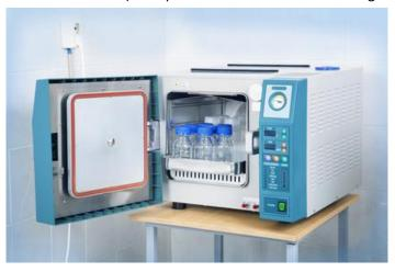
allows inserting them inside the camera alongside with the necessary products, equipment or instruments (all made of materials resistant to high temperatures, e.g. heat resistant glass or stainless steel) undergoing the sterilization.
