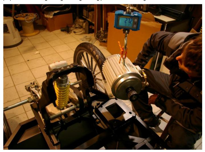
Our target is to design a vehicle which is a true lightweight, with a weight of approximately 350 kg and a small rechargeable battery pack. An additional rechargeable battery will increase its reach considerably. This type of rechargeable batteries which will add an additional weight of 100 kg to the vehicle, can be integrated optionally, which means that they do not necessarily have to be included.
