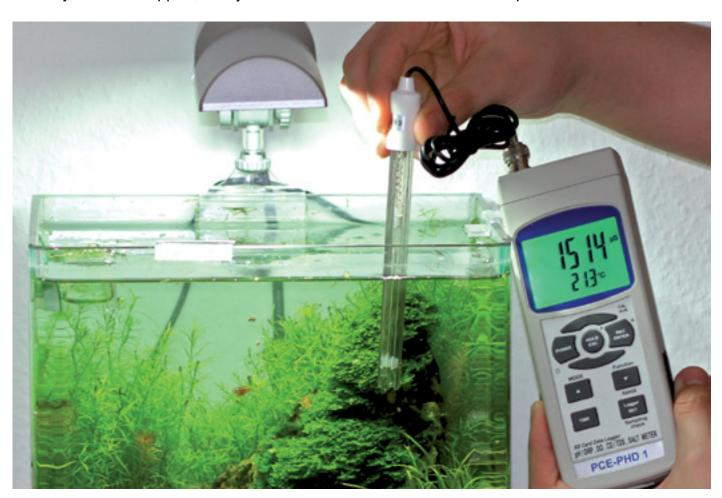
The main unit of measurement is S/cm (µS/cm, mS/cm) for conductivity, ppm for TDS, % for salt content and mg/l for Oxygen content. For highest accuracy of data received, conductivity meters may have temperature compensation, as temperature can have influence on the chemical properties of water.
