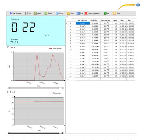
To set the read interval, click on "Option" and then select "Read interval(sec). In the next window, you can set the interval in seconds.
