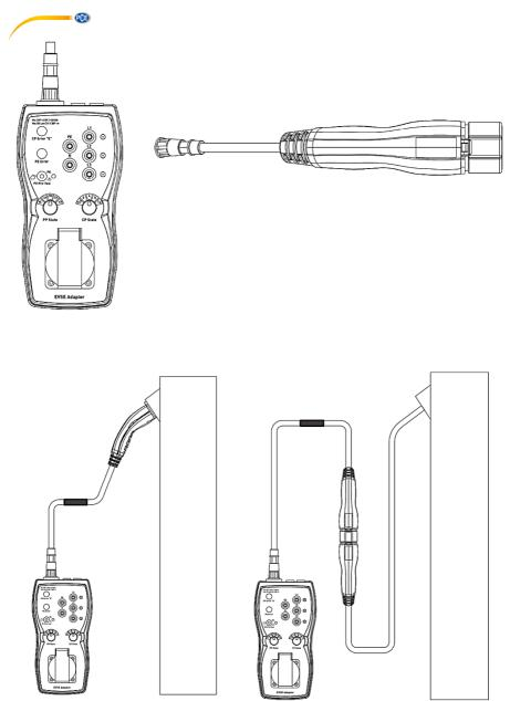
Direct connection to the charging station and connection via a permanently installed cable at the charging station.
