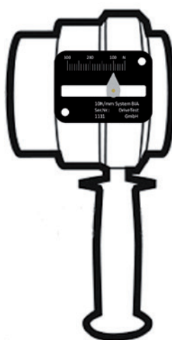
Analysis via mechanical trailing pointer concurrent with measurement
