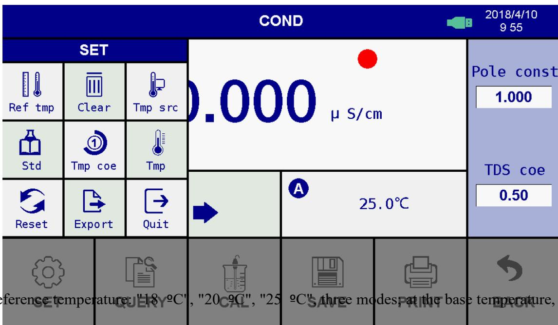
a) Reference temperature: "18 °C", "20 °C", "25 °C", three modes at the base temperature, enter the
