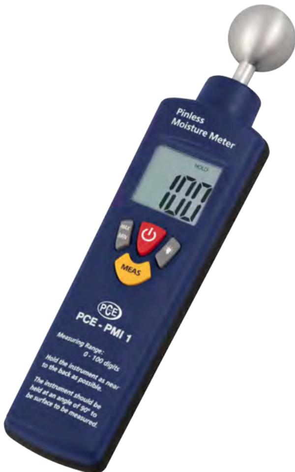
The NON-Contact Moisture Meter is an electronic dampness indicator with a measuring process working on the principle of high frequency measurement. The instrument is used for non-destructively tracing dampness in building materials of all kinds as well as for detecting damp distribution in walls, ceilings and floors. It is particularly suitable for pre-testing the readiness of building materials for covering prior to CM measurement.
