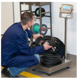
Two range - Parcel Scale / higherresolution / counting function/ sum function/ detachable tripod / battery / container weighing function/ bidirectional RS232 interface
