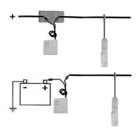
Press and hold down the measurement key on the receiver and follow the signal and thus the cable with the sensor.
