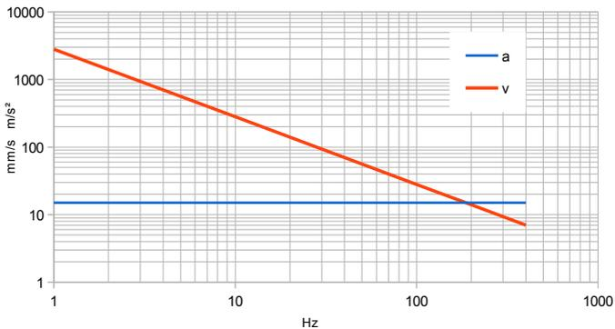
Figure 22: Overload limits for acceleration (a) and velocity (v)
