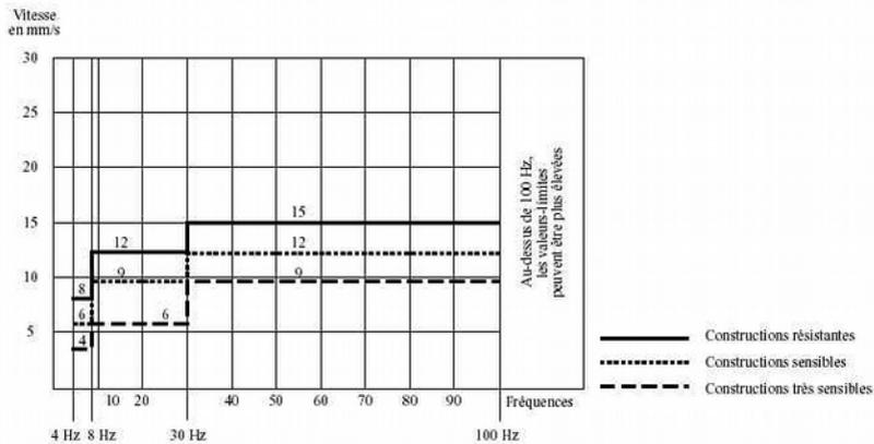
Figure 17: Limits for short-time vibration (Circulaire 23/07/86)
