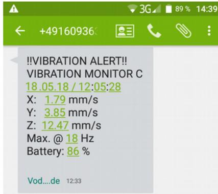
Figure 49: Example of received SMS message
