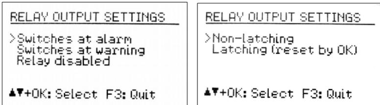
Figure 38: Relay output
