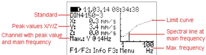
Figure 8: Measurement value display in accordance with DIN 4150-3
