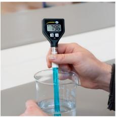
The meter is powered by three LR44 (AG13) batteries which can be easily replaced if necessary. At ambient temperatures between 0 and 50 °C, the measured values are automatically compensated by the built-in temperature compensation. The light and handy pH meter is therefore not only suitable for measurements on samples in the laboratory but also for outdoor use.
