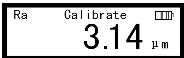
Put the instrument in the scribed line area. Sensor taxiing direction perpendicular to the scribed line of texture direction. Press the Start Key to exit the status of Calibration. Repeated calibration could improve precision.
