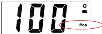
3. Use the "PRINT / UNIT" key to switch between the numbers 5 / 10 / 20 / 25 / 50 / 75 and 100. Select the number that matches the reference number you are using and confirm it with the "COUNT / ENTER" key. The number stops flashing and the scales are now in counting mode. (see picture)
