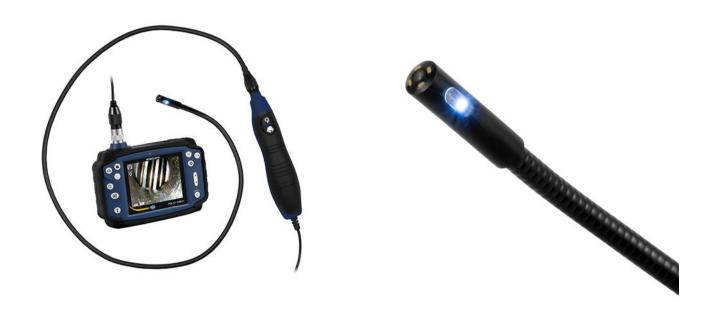
PCE-VE 200SV3 Inspection camera for non-destructive machine diagnosis / Side view camera / Camera head diameter: 9 mm (0.4 in) / 3.5" LC display / 2600-mAh battery / Cable length 3 m (9.9 ft)/ Card slot for micro SD card
