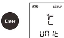
3. Press CAL key to select the temperature unit (°C or °F) and press ENTER key to confirm. The tester goes to temperature calibration mode, the display shows "°C/CAL".
