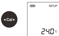
5. Press CAL key to set temperature value and press ENTER key to confirm. The tester shows "YES/HOLD" indicating that the auto-hold function is enabled.
