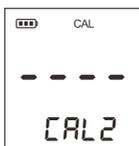
3. Dip the electrode into the calibration solution, the tester automatically shows current calibration standard (e.g., 12.88mS/cm).
