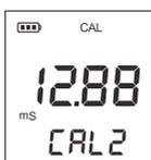
4. Press ENTER key, the default calibration value begins flashing.
