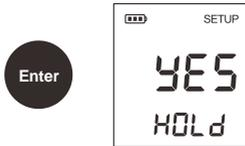
If the auto-hold function is enabled, the tester will automatically sense a stable endpoint reading and freeze it. If you disable this function, the tester allows the user to freeze the reading by pressing the HOLD key.
