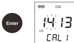
1.6 Press ENTER key to start the calibration. Wait for the reading to stabilize, the display shows "END". The tester returns to measurement mode automatically. Single point calibration is completed.
