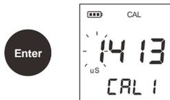
1.5 Press CAL key to set each digit, press ENTER key to confirm. When the setting is done, ensure the displayed value matches your calibration standard.
