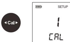
2. Press CAL key again to select 1, 2 or 3 point calibration and press ENTER key to confirm. The tester goes to temperature unit selection mode, the display shows "°C/UNIT".
