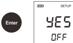
When the auto-off function is enabled, if you do not press any keys for 8 minutes, the tester will automatically turn off to conserve energy.
