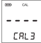
2. Repeat the above steps until the display shows "END", the tester returns to measurement mode. Calibration is completed.
