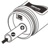
3. Align the slot on the electrode module, push the module into the tester. Twist the electrode collar clockwise until it is tight.
