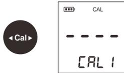
1.3 Dip the conductivity electrode into the calibration solution, the tester immediately shows current calibration standard (e.g., 1413 $\mu$ S/cm).
