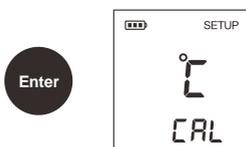
4. If you do not want to perform temperature calibration, press ENTER key, the tester goes to the next option. If needed, press CAL key to enter the temperature calibration mode, the display shows current temperature reading.
