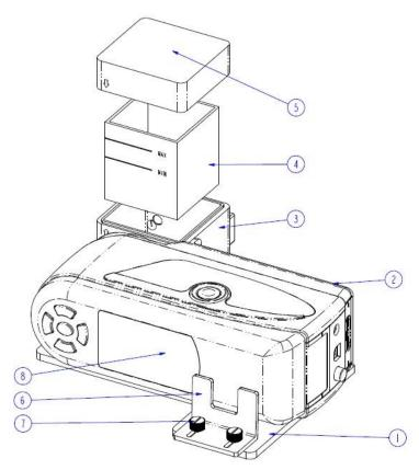
Fill the tank (4) with the desired medium and put it into the measuring chamber (3). Make sure
