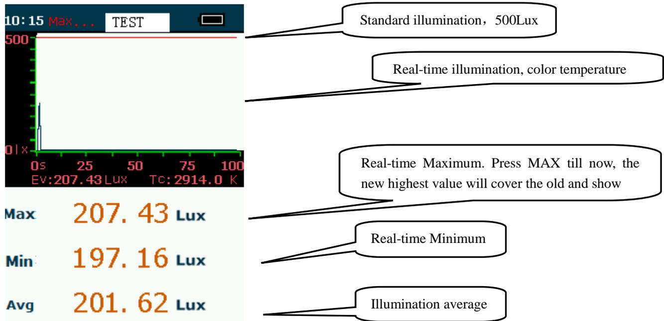
Under the “MAX” condition, Press the ‘HOLD’ key, the device stop measuring and keep the screen still, then give the tips about the appearing time of Maximum and Minimum value. See as followed:
