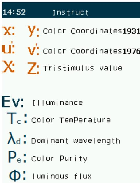
The definition of photometric and colorimetric symbols are provided in the page for operation.
