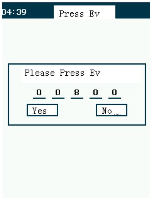
This function sets a standard illumination value. After entering this screen, press UP/DOWN button to firm a number within 0-9. After completing a set, cursor will move to another position to choose. Completed five blank positions setting, press UP/DOWN button to choose the weight of issue, or re-input a standard illumination value.
