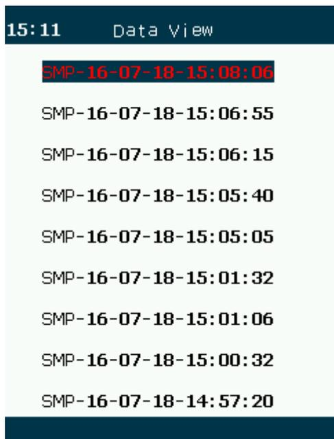
Data list is sorted by time, and device only stores latest nine data. New data would cover previous data automatically.
