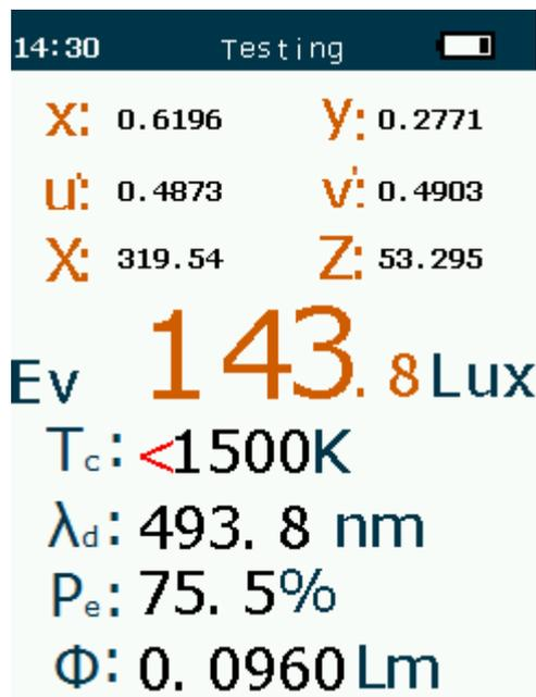
Measuring screen shows all real-time measured values, can be easily seen the measured Light Source parameter values.
