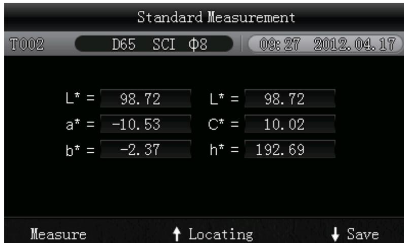
A reading which has been determined by using the “Standard Measurement” automatically serves as a reference value. You can add one or more sample measurements to this reading. To do so, you have to switch to the “Sample Measurement” screen:
