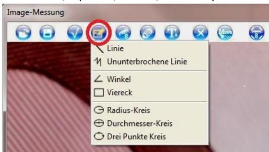
Perform measurements after calibrating the microscope. Choose a suitable object and mark the measuring points in the image. The measurement result is displayed. By clicking the mouse in the result, the image can be drawn.
