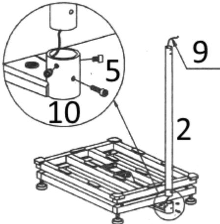
Now the cable (9) must be guided through the tube-display holder (6) and then through the U-shape display holder (4).
