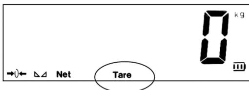
**ATTENTION:** The weighing range is not increased by taring, so if you have a 30 kg scale and tare 10 kg, you only have a weighing range of 20 kg left.
