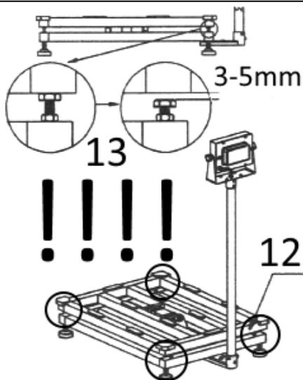
Finally, the balance must be aligned horizontally. To do this, turn the adjustable feet (14) of the weighing platform until the level indicator (15) shows a level position and the balance stands stably.
