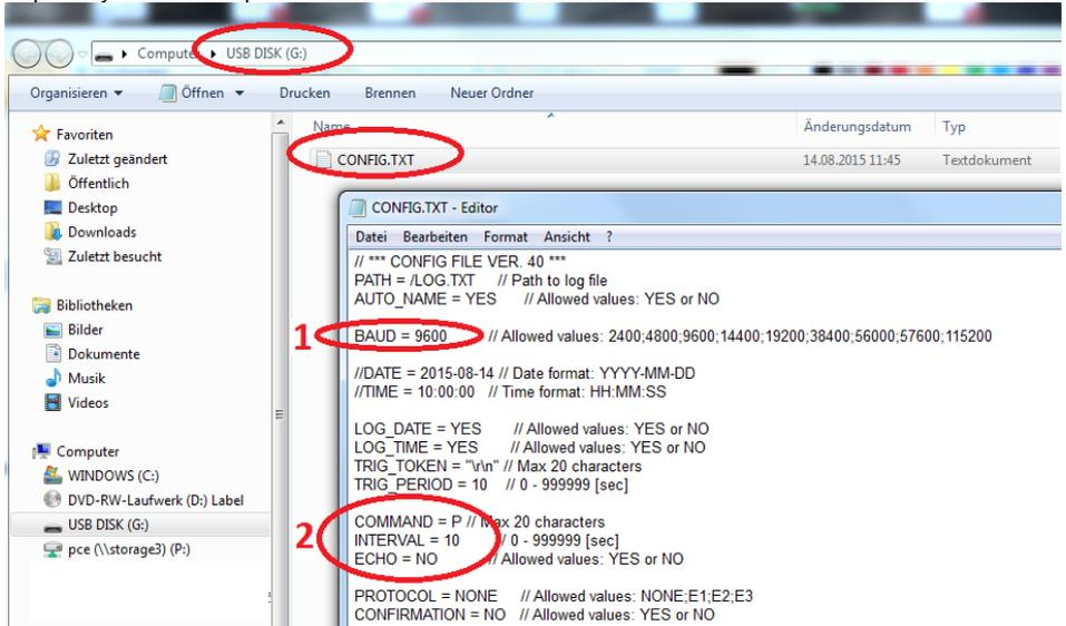
1. You have set the baud rate in the balance to 9600, so the baud rate here must also be 9600. Please adjust if necessary.
