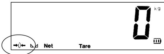
If you wish to have the existing weight displayed after starting the scales, as is useful for weighing containers, for example, some items must be changed in menu mode (see menus C07 / C08 / C09 and C05 to determine the internal zero point).
