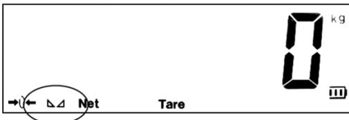
If the balance does not respond, check the power supply to the display. If the stability symbol does not appear, check the base and level the balance.
