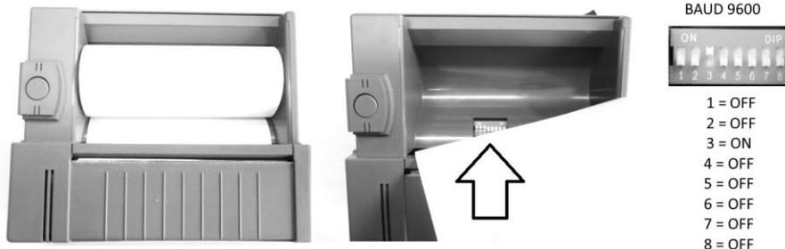
Then connect the printer to the display of the balance via the RS-232 interface.
