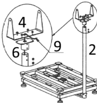
The display (3) must now be screwed onto the U-shape display holder (4). The inclination of the display can be varied with the adjusting screws.
