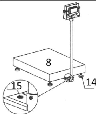
**After setting up the platform scales, check the gravitational range of the place of installation in the scales. You will find this function in the internal menu under "C37.**
