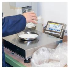
The dual-range scales of the PCE-EP P series are suitable for a wide variety of applications in laboratories as well as in industrial and commercial enterprises due to their robust construction and the diverse setting and evaluation functions. The advantages of this series also include great flexibility when it comes to the installation and a freely adjustable measuring unit for special applications.
