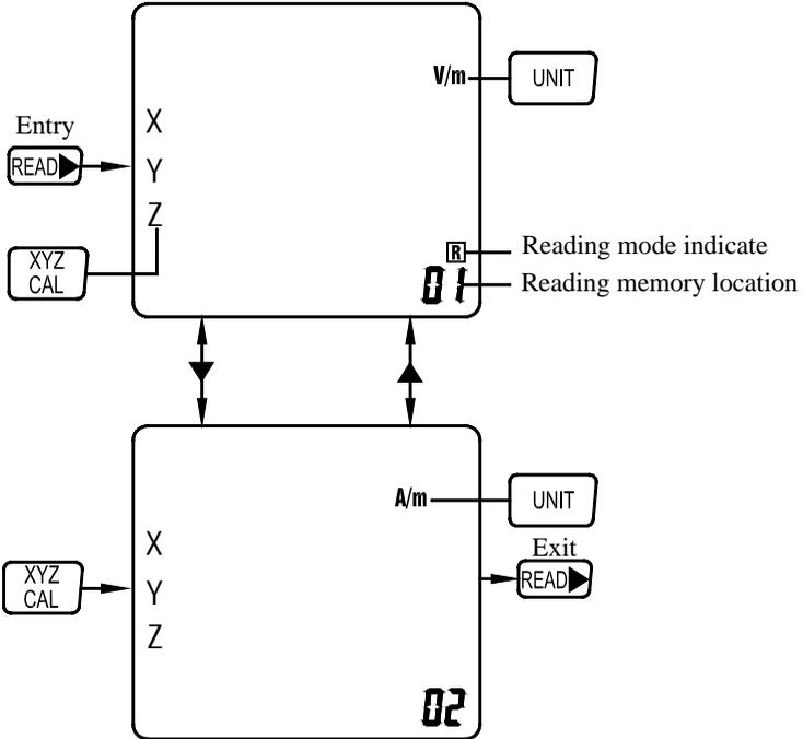
1. Press **READ** key, the display then shows "**R**"(reading mode).
