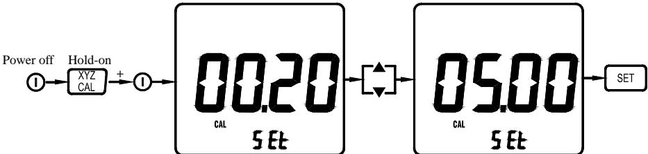
When the meter is normally turned on, the calibration factor set value will display for 2 seconds.
