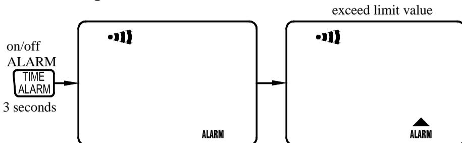
1. Press **TIME ALARM** key for 3 seconds to switch the alarm function on or off. The “ALARM” and “**•••**” symbols in the display indicates that the alarm function is on.
