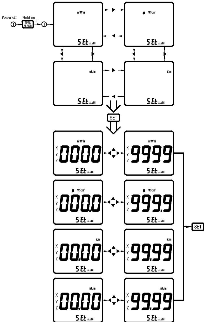
When the meter is normally turned on, the alarm set limit value will display for 2 seconds.
