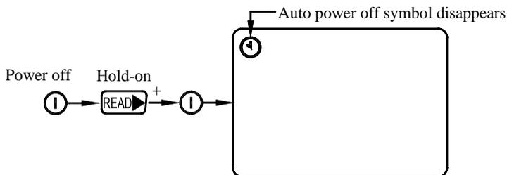
When the meter is normally turned on, the auto power off function is on.
