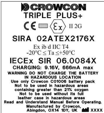
1. The equipment is Category 2G and may be used in zones 1 and 2 with flammable gases and vapours with apparatus groups IIA, IIB & IIC and with temperature classes T1, T2, T3 and T4.
