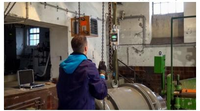
displayed in the units kilogrammes, lbs, Newtons, kilonewtons and tonnes. The values can be saved to the internal memory for later evaluation. The PEAK function makes it possible to determine the maximum value of fluctuating values from individual measurements with a sampling rate of 2.5 hertz. The hanging
