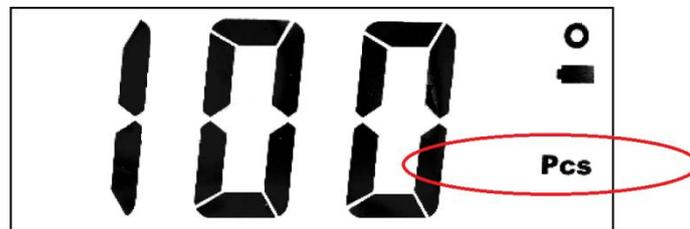
You can switch by means of the “**Count / Enter**”- key between count mode and standard mode. The determined weight per piece will be saved until the next alternation.
