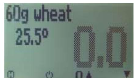
6. Fill up the cup with the sample material (+/- 0.5g). The filling quantity needed is shown on the upper left corner on the display of the device.
