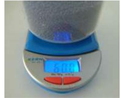
7. Fill up the measuring device with the sample material. The filling needs to be done slowly and constantly to ensure reproducible results. There must not be used a funnel or anything similar for filling.
