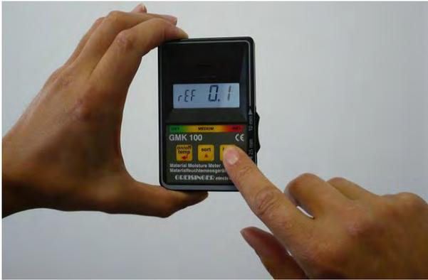
It is recommended to run regularly the zeroing function for best measuring results:
