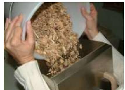
8. Remove material till the next lower weight range is reached. If only a little missing (e.g. 0,10kg) to the next higher level, it should be filled up to that stage. The actual weight is shown on the scale.
