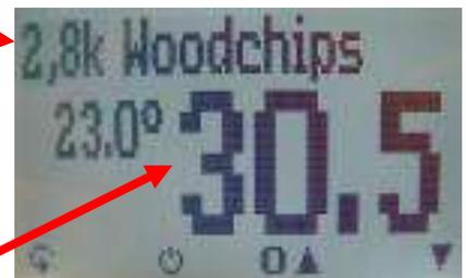
11. If the measure value is blinking, the valid measuring range is exceeded (limits see list on page 5). In this case the accuracy will be decreasing. If you are measuring wood chips, select the next higher weight class and refill wood chips to reach the higher filling weight.
