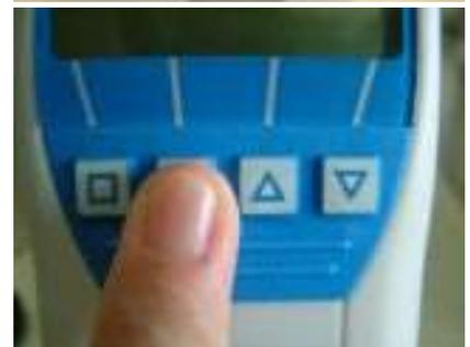
4. Switch on the moisture analyser BM1 by pressing the power button (⏻) for 3 sec.
