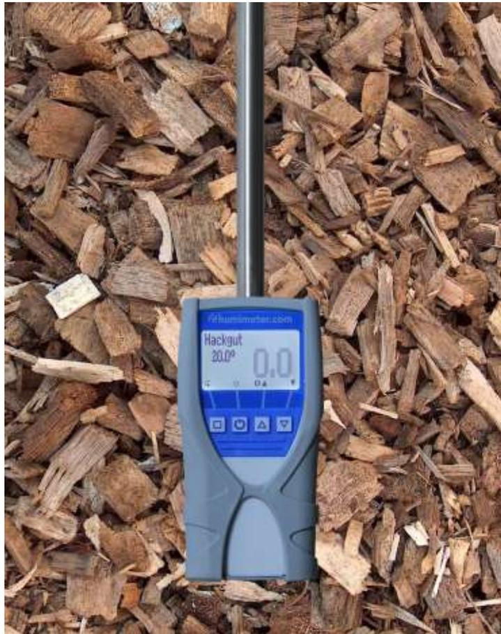
Moisture meter with insertion probe
