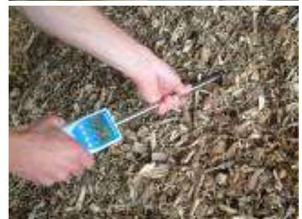
4. Plug the probe of your moisture analyser BLL **straight into the wood chips**. It is **not allowed to load the measuring head incorrect or drop it down!**
