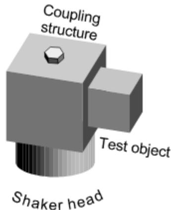
Please note that heavy connecting cables should be supported close to the test object. However, an application of force via the cable must be avoided. The maximal torque rating of **1 to 2 Nm** at the vibration exciter must not be exceeded since this may damage the instrument. The PCE-VC20 should be placed on a rigid surface. Hand-held operation is not recommended because of possible errors.
