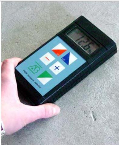
A hand holds the FMW-B moisture detector against a grey concrete surface. The LCD screen displays '12.6%'. |
