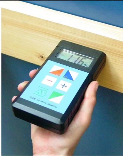
A hand holds the FMW-T moisture detector against a horizontal wooden surface. The LCD screen displays '11.6%'. |
