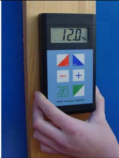
A hand holds the FMW-B moisture detector against a vertical wooden surface. The LCD screen displays '12.0%'. |
