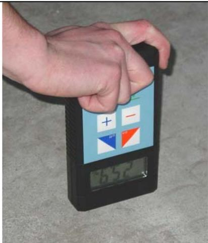
A hand holds the FMW-T moisture detector against a grey concrete surface. The LCD screen displays '6.5%'.    |
