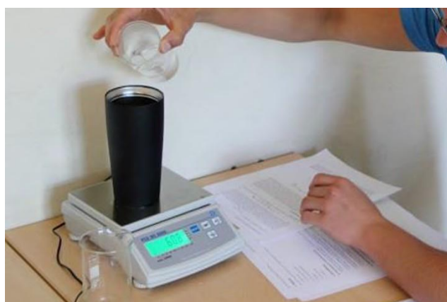
Fig. 3 – A student determining the heat capacity of the alcohol
