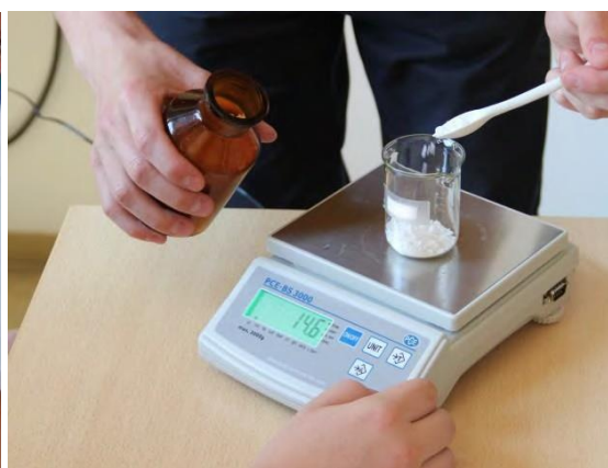
Fig. 4 – A student is weighing \text{CaCl}_2 , the solution heat of which should be determined
