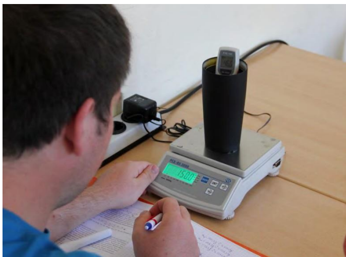
Fig. 2 – Determination of the calorimeter constant of the thermo cup
