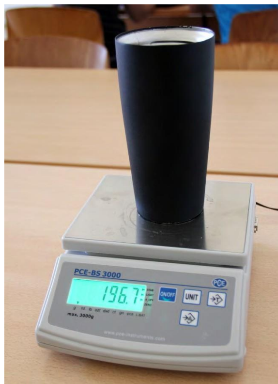
Fig.1 – Determination of the ice fusion heat with the help of the analytical scale PCE-BS 3000
