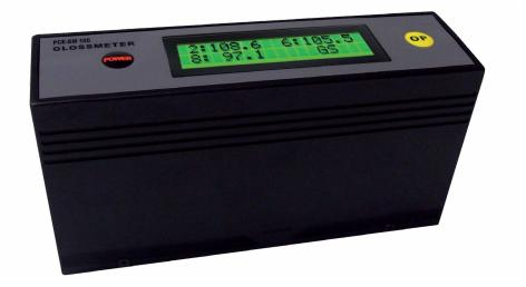
low gloss surfaces, where the measurements value will be less than 10 GU – then the gloss meter angle should be 80°.
