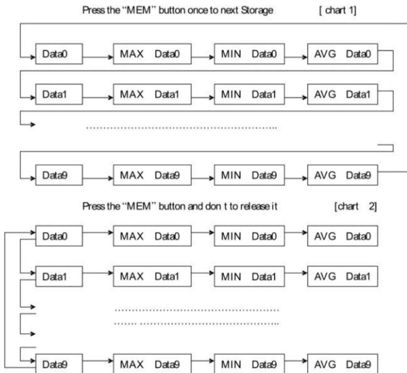
\* **Measurement Mode Switch:** Release the "MEAS" button and press the "MODE" button before the instrument auto power off(released the "MEAS" button this instrument will auto power off in 15 sec). There are two group of measurement. You can press the "MODE" button once to change from RPM,rpm,HZ,...to the next sequentially. Press the "MODE" button and hold for
