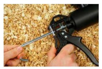
6. Use the compacting device again to push out the sample.
