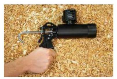
After operating the compacting device a couple of times, an indicator will show up to give information on the compression pressure. The appropriate compression is reached when a red ring around the indicator is shown. The red ring should only point out of the head of the measuring chamber by a maximum of 0.5 to 1 millimetre.
