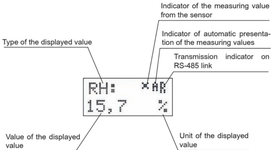
*Fig. 7. Description of the P18D transducer readout field*
