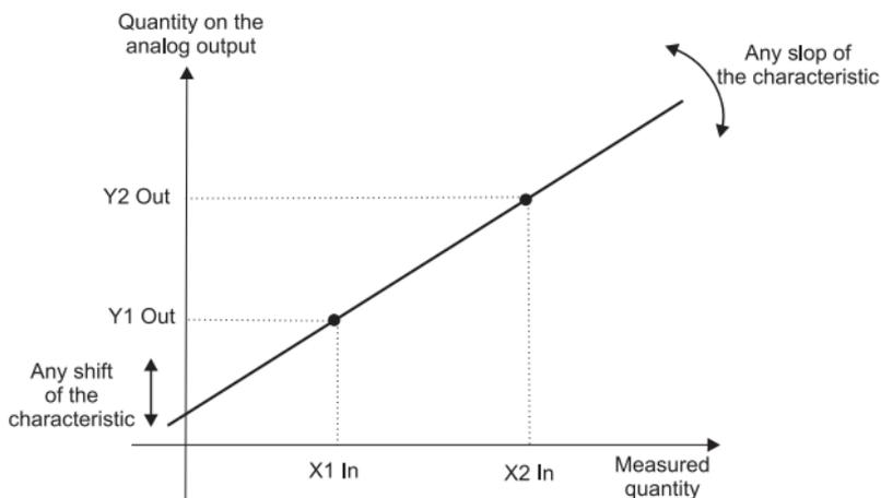
Fig. 11. Individual characteristic of analog output
