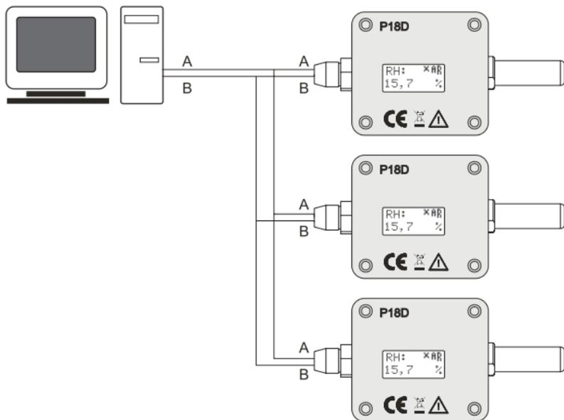
Fig. 13. Connecting the RS-485 interface.
