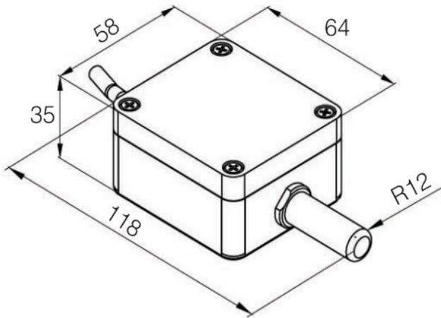
Fig. 3. Overall dimensions of the P18(D) transducer
