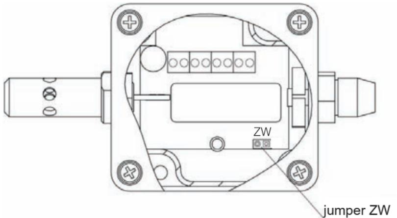
*Fig. 13. Placement of the jumper setting temporary communication parameters*
