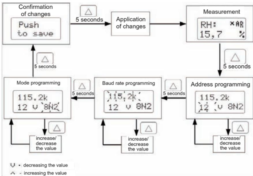
Fig. 10. Programming parameters algorithm of the P18D transducer
