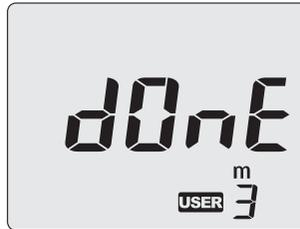
**Note:** If the display shows "FAl L", and "ERROR", the setting fails and you should check whether the connections and contacts are correct and good. If press the **CAL** Button again, the meter will return to measurement mode.
