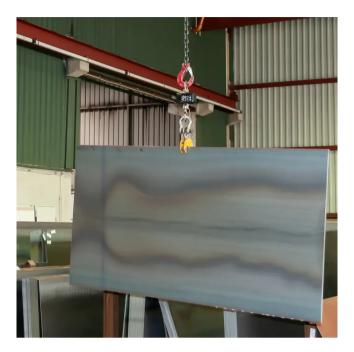
Crane scales with a measuring range of 0 ... 1000 kg / Backlit LC display / Battery operation / Robust metal housing / "Hold", "Tare" and "MAX" functions / Various mass units / Incl. ISO calibration certificate
