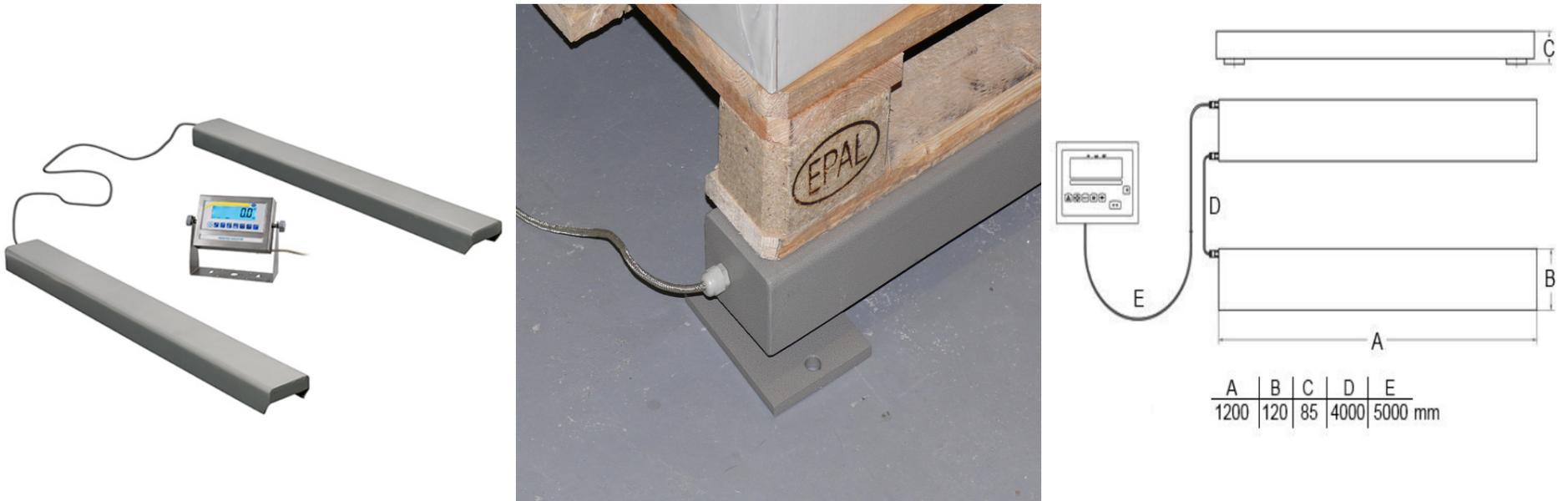
PCE-SW 5000N is a portable battery-powered industrial pallet scale or floor scale featuring two heavy-duty parallel weighing beams made of lacquered steel that can be positioned up to 4 m / 13 ft apart. Thus, the adjustable width accommodates multiple pallet, box and container sizes. In addition, the scale's stainless-steel-encased display can be placed up to 4 m / 13 ft away from the weighing beams, allowing for wall mounting.
