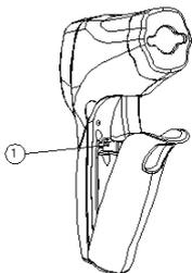
Select the desired temperature unit (°C or °F) using the °C/°F switch ① the location of which can be seen in the picture.
