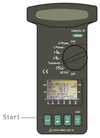
After users press the FUNC button, the LCD will become blank and the LED at the bottom starts to flash.
