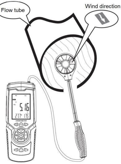
To make a measurement, align the flow sensor with the flow direction. An arrow inside the sensor indicates the orientation in relation to the wind flow. Wait for at least two seconds for the reading to stabilise.
