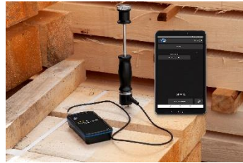
Figure 3 PCE-WMT 200 with measuring electrode
