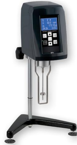
The viscometer has a measuring range of 1 ... 100,000 cP. With an accuracy of  $<\pm 2\%$  of the range, the viscometer is a precise measuring device to determine the viscosity of a sample liquid. The viscosity is determined by the viscometer on the basis of an applied mechanical resistance that acts in the opposite direction to the rotational movement of a spindle. The viscometer can be operated with an adjustable speed in the range between 6... 60 RPM.
