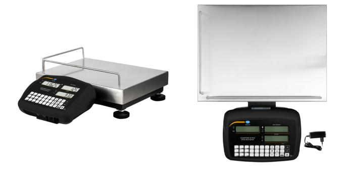
Low-cost benchtop scale up to 150 kg, Readability 10 g, Mains and battery operation, Large 20 mm LC display, Removable stainless steel platform, Zero and tare function
