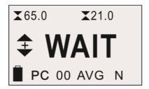
If "I.DLY" is shown on the display, the force gauge will wait until the set minimum time has elapsed.
