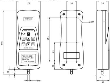
Dimensions for models with external measuring cell
